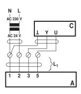
A = Actuator C = Control unit (controlling unit) L1 = Connecting cable of the actuator
