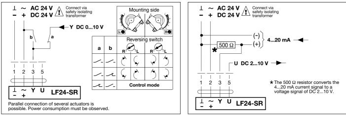
Control by 4...20 mA via external resistor
